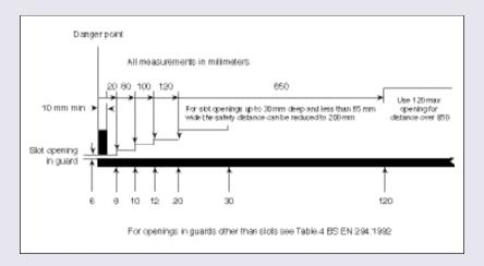
**Example:** If it is necessary to provide an opening between 12 and 20 mm, the guard should be positioned at least 120 mm away from the danger point.
