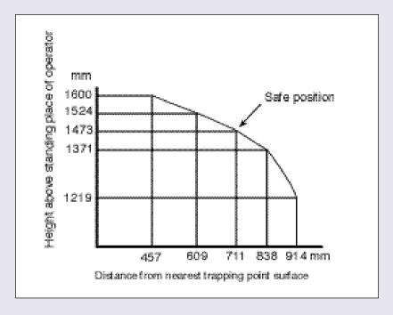
**Example:** When the guard is 1524 mm above the standing position of the operator the trapping surface should be at least 609 mm away.
