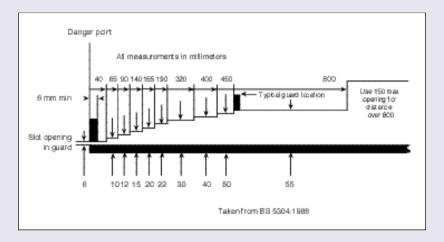
**Example:** If it is necessary to provide an opening 30 mm deep, the guard should be positioned at least 190 mm away from the danger point.
