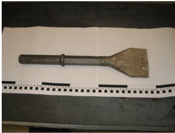
Figure 9a: Standard cutter used for breaking tarmac
