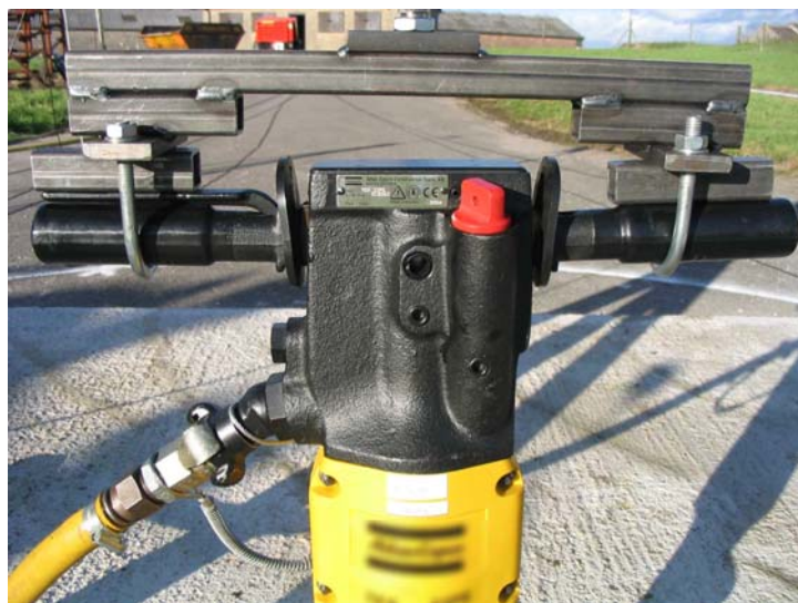
Figure 8: Method used for attaching pneumatic jack to breaker handles
