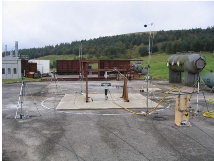
Figure 2: NEEEEOR 2001 standard test rig at HSL for concrete breakers
