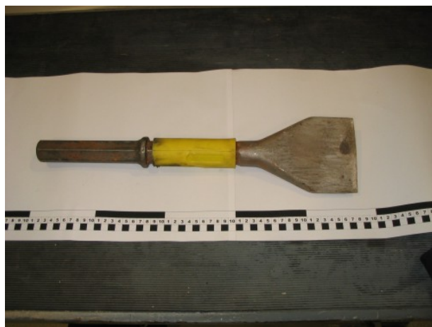
Figure 9b: Vibration reduced cutter used for breaking tarmac
