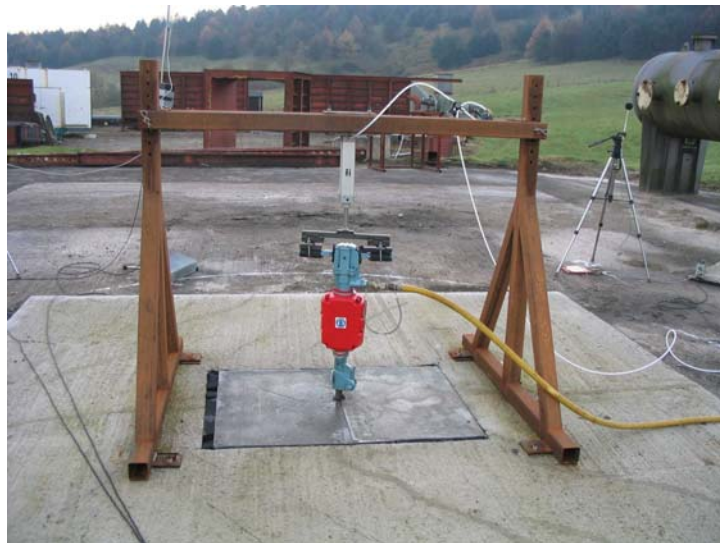
Figure 7: Set up for supporting breaker during noise emission tests
