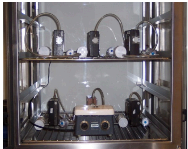
Figure 5 — Environmental setup to compare TCP capturing efficiency
