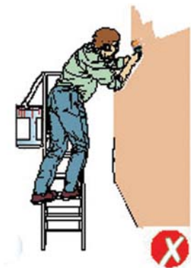
Figure 2a - avoid sideways loading
