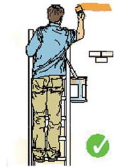
Figure 1b - correct position
