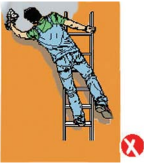
Figure 1a - avoid overreaching
