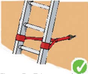
Figure 7 - Tying near the base of the ladder
