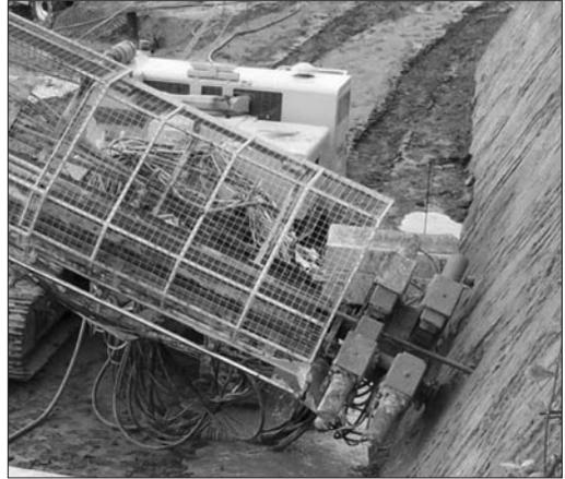
Nota Questa situazione è trattata nella EN 16228-3:2014 al punto 5.12.2, 4° periodo: The manufacturer is not responsible for guarding the drill string beyond the breakout clamps. The area ahead of the breakout clamps of the machine that has exposed drill rod/pipe should be job site controlled
