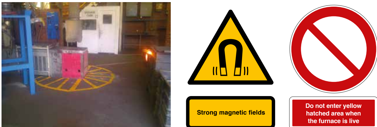
Figure 8.7 — Painted floor and associated warning notice to indicate the area in which the action levels could be exceeded
