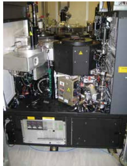
Figure 9.2 — Reaction chambers in the service area
