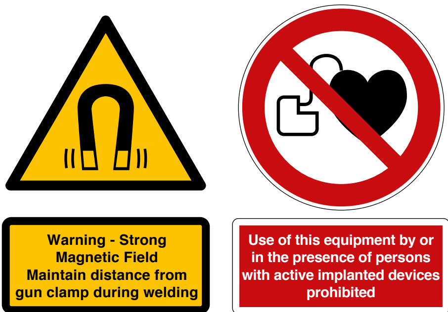
Figure 6.15 — Examples of strong magnetic fields warning notice and a notice prohibiting the use of the welder by, or in the presence of, AIMD wearers
