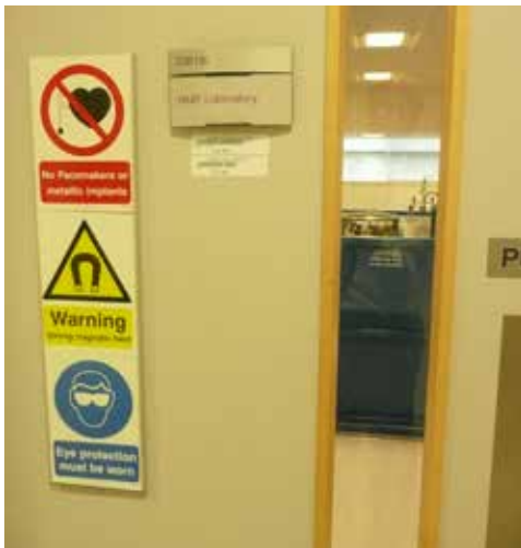
Figure 2.3 — Warning and prohibition notices on the entrance door into the NMR Laboratory
