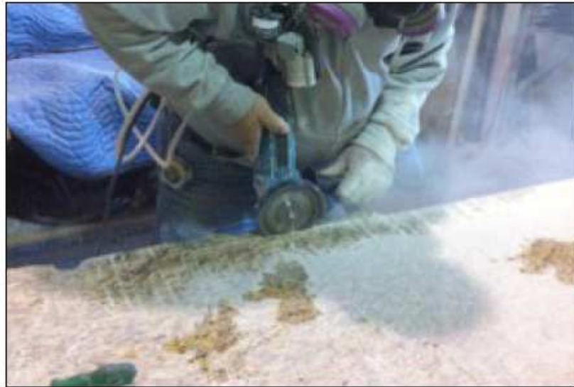
Cutting stone, as pictured, generates dangerous crystalline silica dust that can become trapped in lung tissue and cause silicosis.
