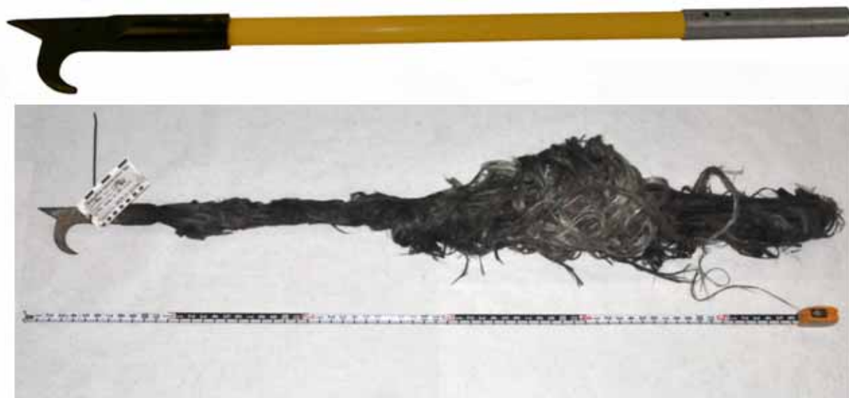
Figure 40. Photo of undamaged 179 (top) and burned during incident (bottom) pike pole used in early attempts to remove 4-sidecut insulation.
