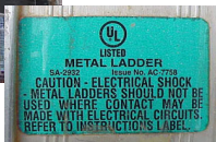
A painter was electrocuted when moving a metal ladder on this jobsite.
