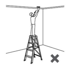
Do not work on the top rung of the ladder.
