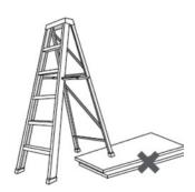
Place the ladder on stable and level ground. DO NOT place it on an uneven surface.
