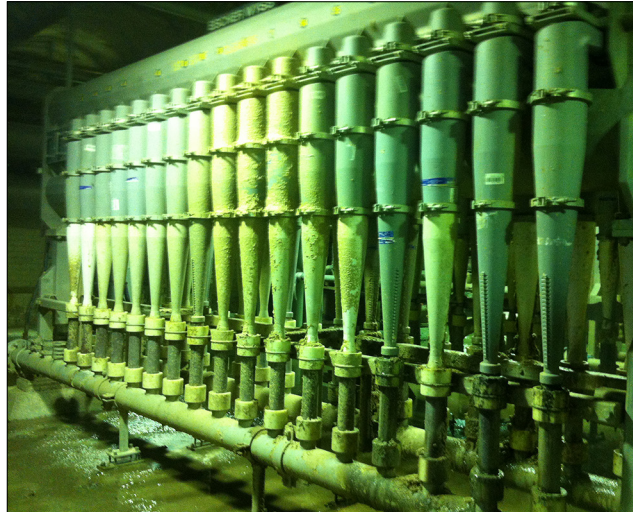
Figure 21 Bank of plastic vortex cleaners with glass sights
