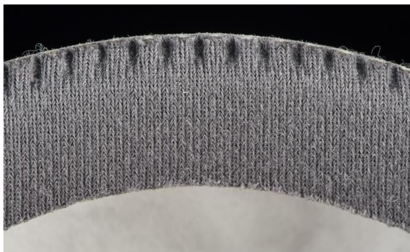
Figure 27 Photograph of an example of a Type 2 faceseal
