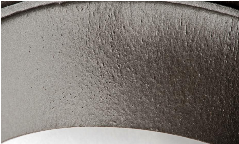
Figure 25 Photograph of face seal F3 after being worn by a test subject with stubble
