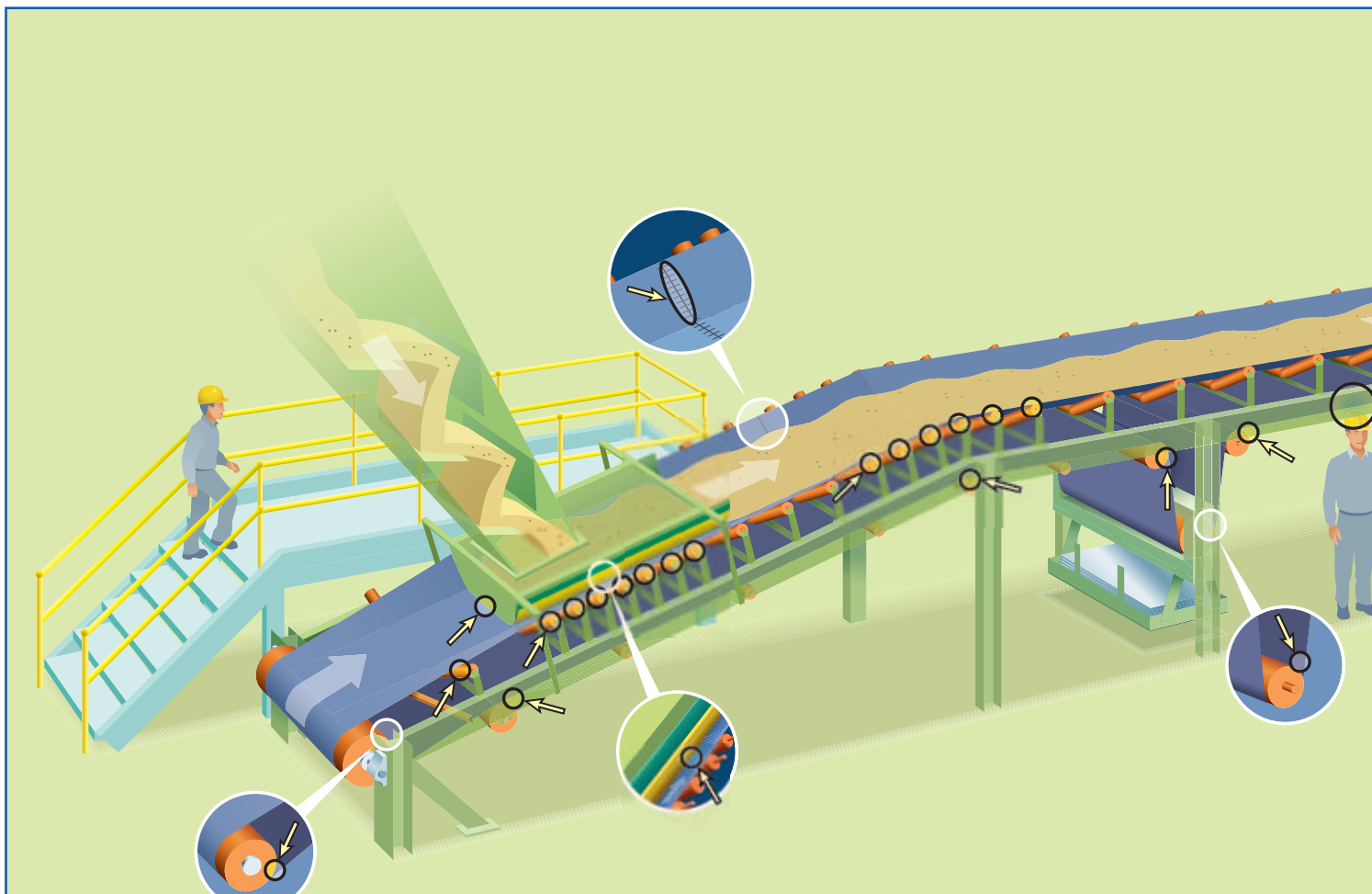
FIGURE 1-6 TYPICAL MECHANICAL HAZARDS
