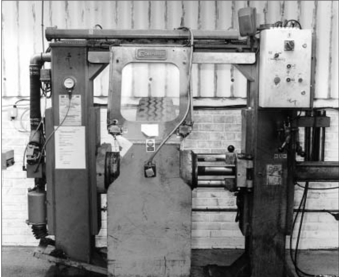
Figure 5 Truck tyre inflation-testing machine fitted with safety guard
