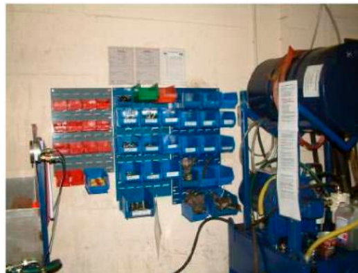
Figure 6 Organising test connectors in a receptacle
