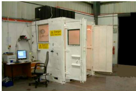
Figure 2 A converted steel container with remote regulation of the test apparatus provides a test booth for various-sized assemblies inside. Pressure indicators inside and outside the booth verify when pressure has been exhausted
