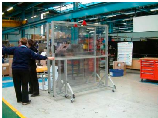
Figure 5 Portable barriers (either single or interconnecting panels) can provide a temporary enclosure for unusual items, but this places high reliance on personnel to ensure there are an adequate number and they are correctly positioned
