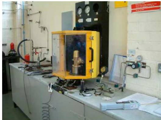
Figure 4 An enclosure for valve testing includes a hinged polycarbonate section with access holes to allow a gas sniffer or soapy water applicator to be inserted inside, to check for leaks
