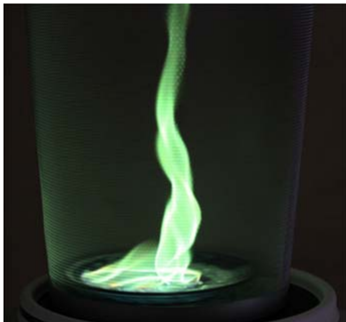
Figure 2. Boric Acid Fire Tornado with methanol 6
