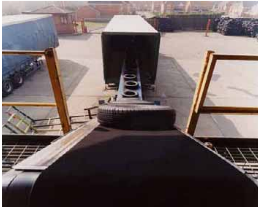
Figure 9. Conveyor feeding retreads into delivery vehicle.
