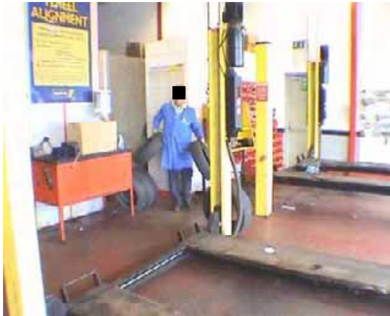
Figure 4. Sometimes tyres are carried through the fitting bay, in which case a carrying assessment should also be made.
