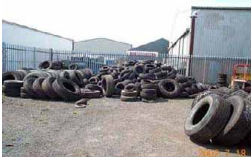
Figure 16. Bad practice. How not to store used tyre casings!
