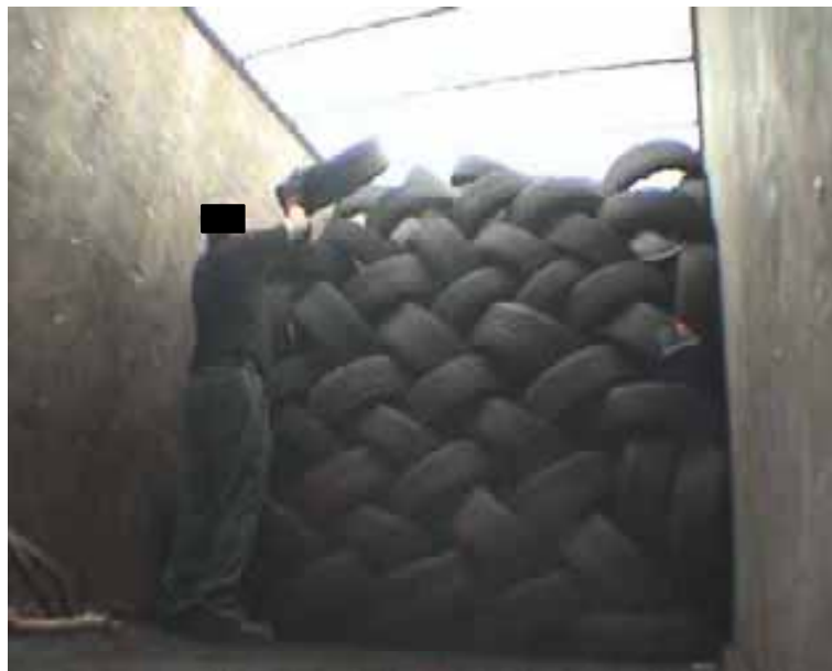
Figure 5. Lacing the casings inside the collection vehicle. A roof letting in daylight like this one makes the job easier.
