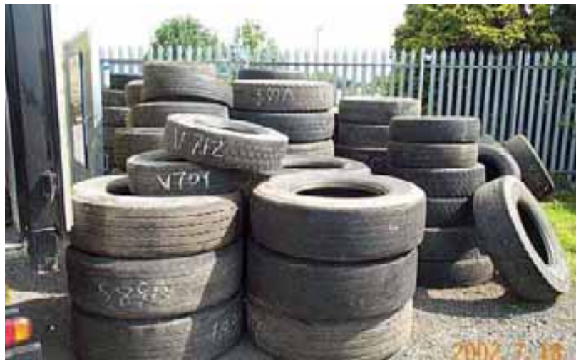
Figure 15. Bad practice. Large tyre casings stacked horizontally. They now have to be lifted off and turned to the vertical for rolling to the collection vehicle.
