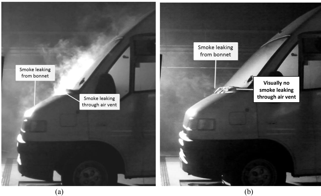
Figure 4.3 – Screen grabs of smoke leaking from the van’s bonnet a) with the ventilation set to fresh air intake mode b) with the ventilation set to recirculating mode
