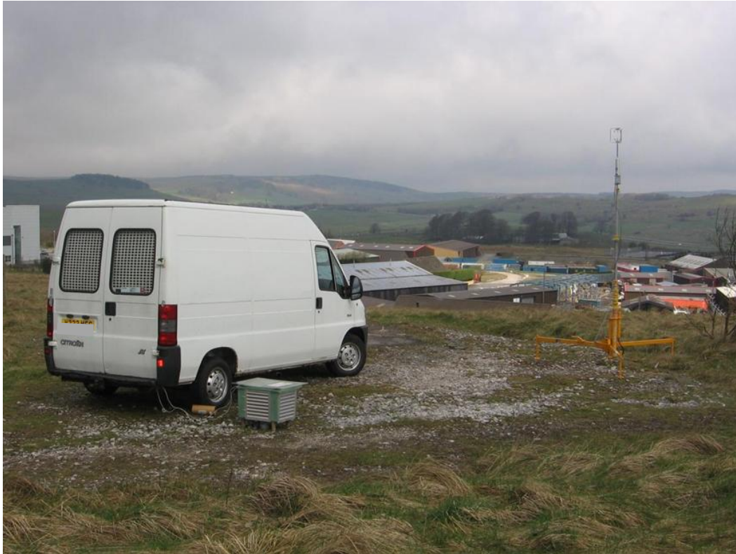
Figure 3.4 – Photo of the test vehicle parked in an exposed location. The ultrasonic anemometer can be seen to the right of the picture.
