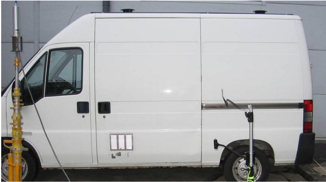
Figure 3.6 – Test vehicle showing wind powered rotary ventilators and side grille vents
