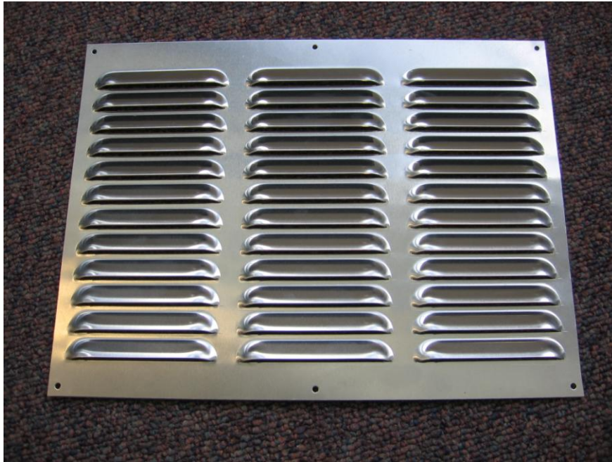
Figure 3.6 – Photograph of the ventilation grille. These were fitted at two locations on the outside and inside of the vehicle
