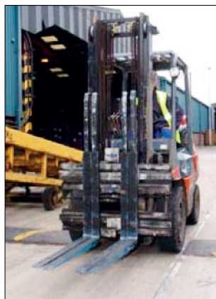
Figure 3 A lift truck passing through an interrupted speed hump
