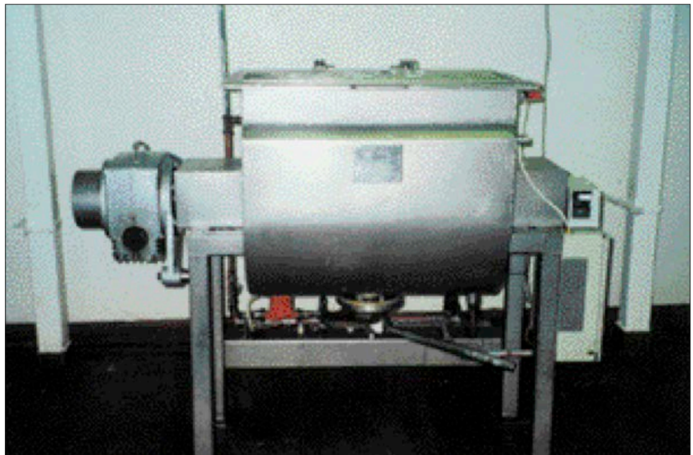
Solution: mixing machine for fondant and chocolate
