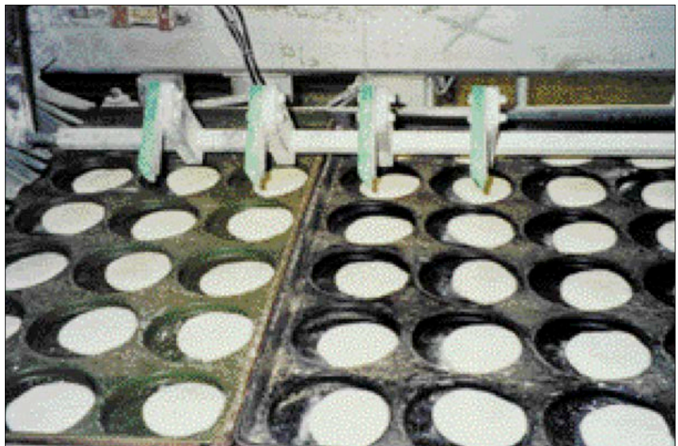
Solution: tray-indexing arm with plastic-capped fingers
