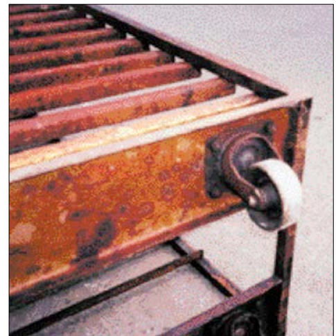
Problem: rack fitted with original metal wheels
