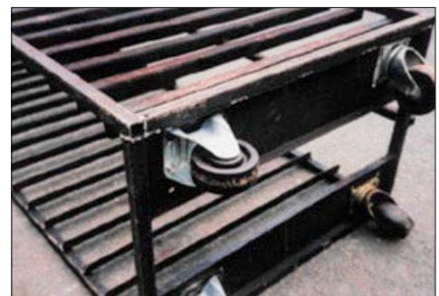
Solution: rack with new phenolic wheels
