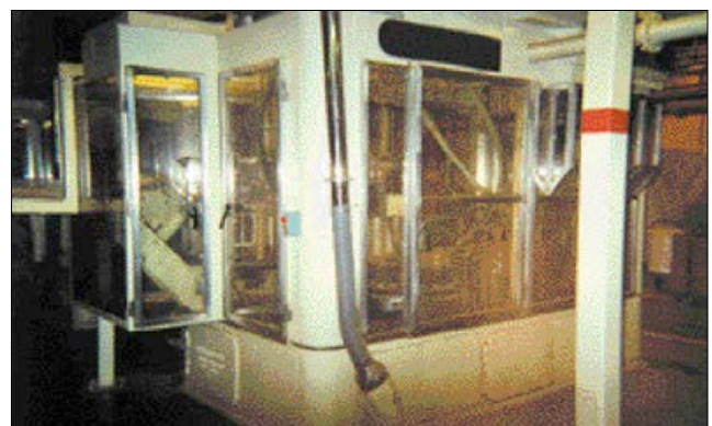
Solution: new sealed enclosure for cup-filler machine
