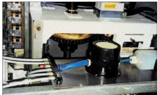
Solution: new, quieter water pump
