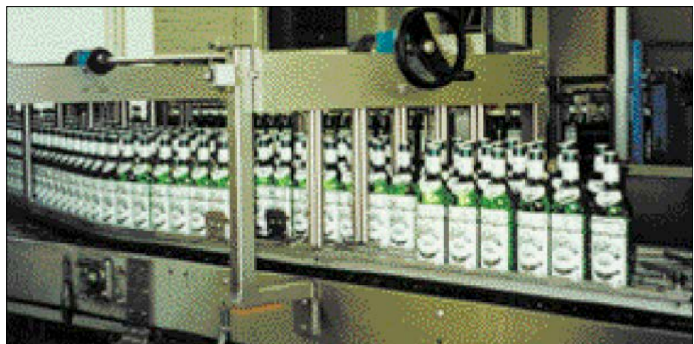
Solution: new variable-speed conveyor with adjustable guide-rails
