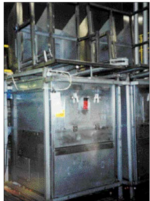
Solution: stainless-steel cap-hoppers inside new segregated enclosure
