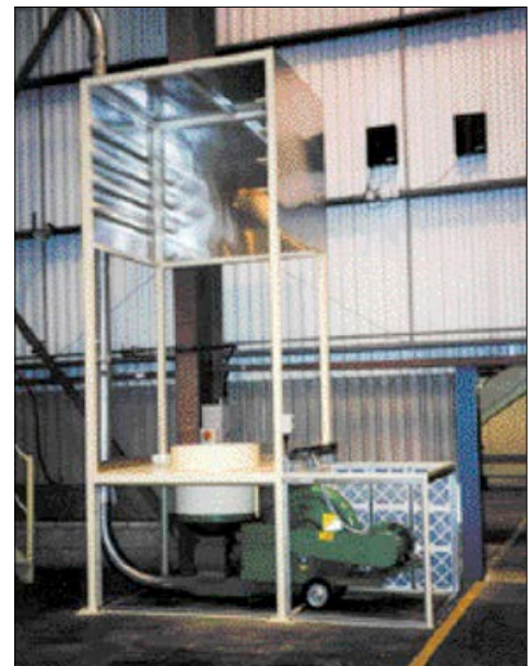
Solution: new blower machine installed in enclosure (sound-absorbent side panels removed for clarity)
