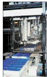
Solution: new robot installed to change tins
