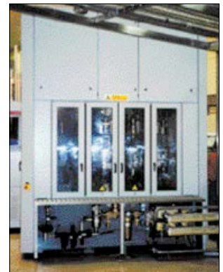
Solution: new bay lined with acoustic panels for enclosed bottle-blowers
