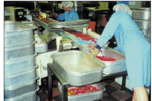
Problem: sweets dropping into metal trays causing noise
