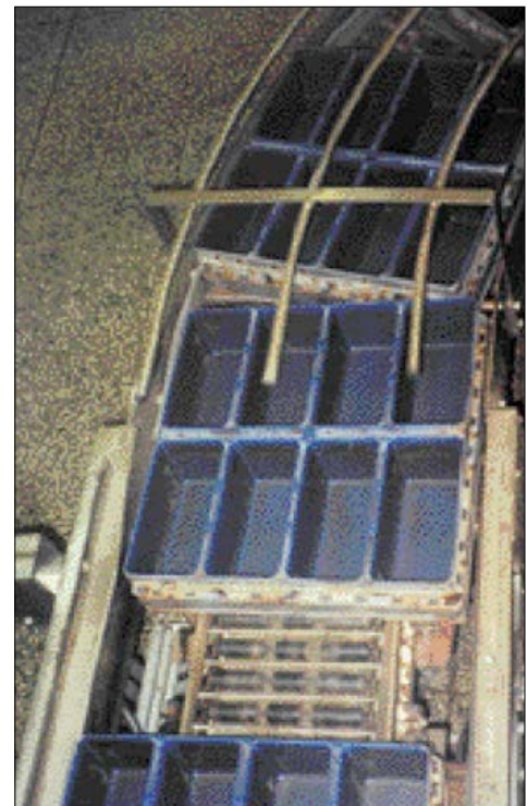
Solution: new conveyor fitted with freely rotating rollers (visible between blue tins)
