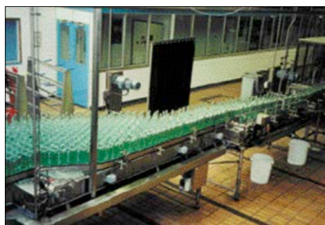
Solution: new design of conveyor and accumulation table
