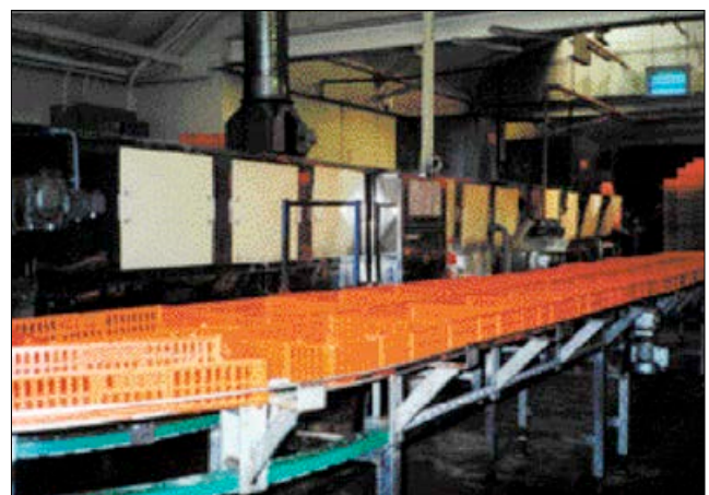
Solution: basket-washing machine in use
