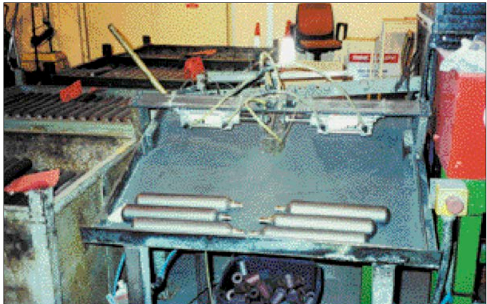
Solution: steel table covered with rubber matting to reduce impact noise
