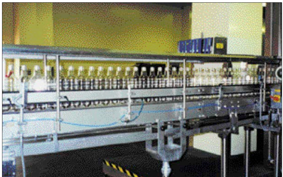
Solution: new machine fitted with guide-rails in laner mechanism
