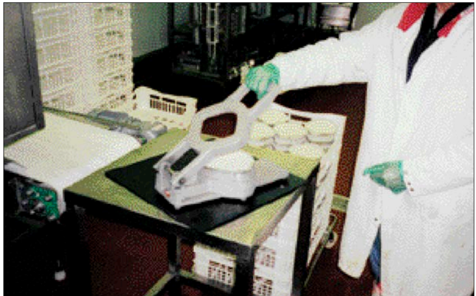
Solution: hand-operated crimping machine mounted on layers of rubber
