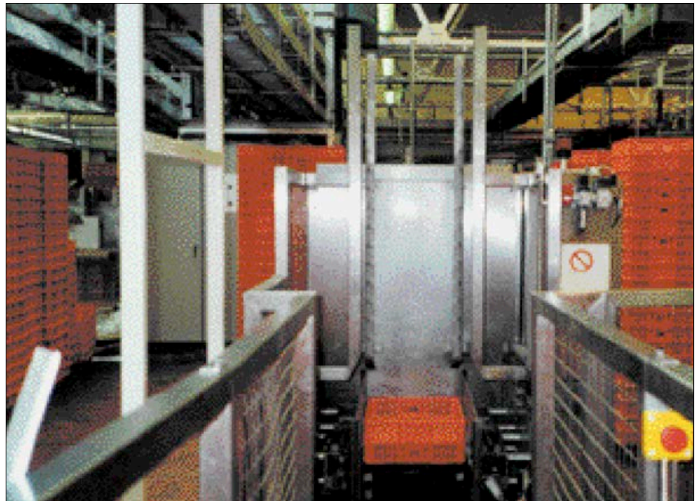
Solution: bread-baskets in stacking machine
