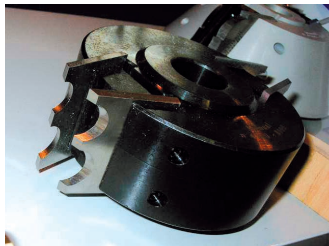
Figures 1a & 1b Round form tool with limited cutter projection
