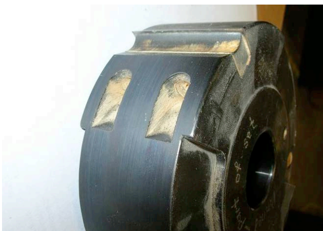
Figure 7 Key or wedge-shaped cutter
