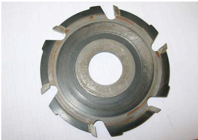
Figure 4 Example of a non-round form tool with limited cutter projection
