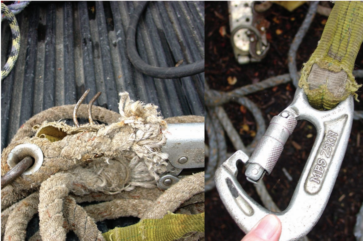
Before you use a personal fall-arrest system, inspect components for damage or wear.
