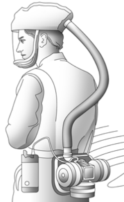
Loose-Fitting Powered Air-Purifying Respirator (PAPR) APF=25
