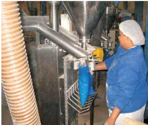
Fig. 4. Garlic dust exposure during milling, blending and packing procedures in a spice mill.
