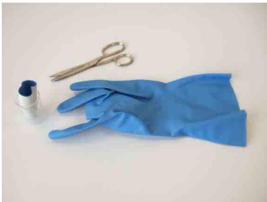
Figure 2.1 Experimental set up for 4-hour continuous contact screening test featuring: inside-out finger of glove placed upright in a beaker. The test liquid is pipetted carefully into the inside-out finger of the glove
