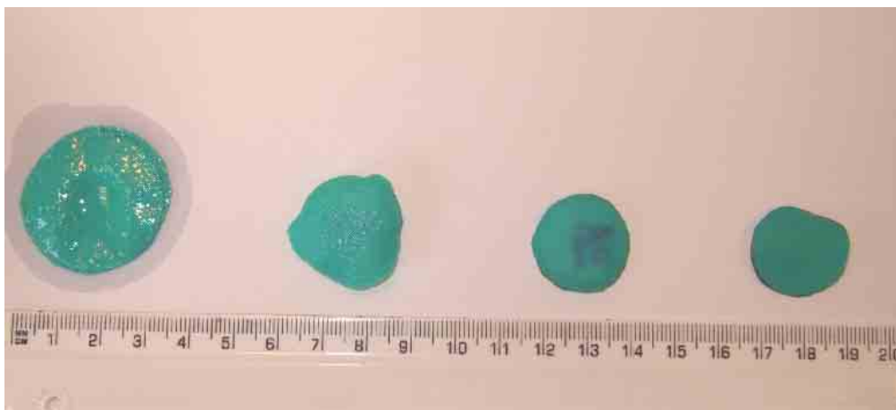
Figure 3.14 Solvent-swollen reusable Solvex nitrile glove material (B), pictured after 8 hrs of continuous contact with (left to right) NMP, GC300, DSI 6000 and no solvent. The NMP swollen sample is surrounded by solvent that it has sweated out following its removal from the test rig
