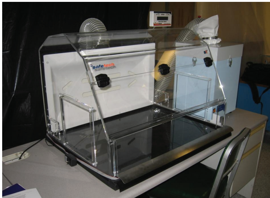
Figure 10. Nano containment hood adapted from a pharmaceutical balance enclosure
