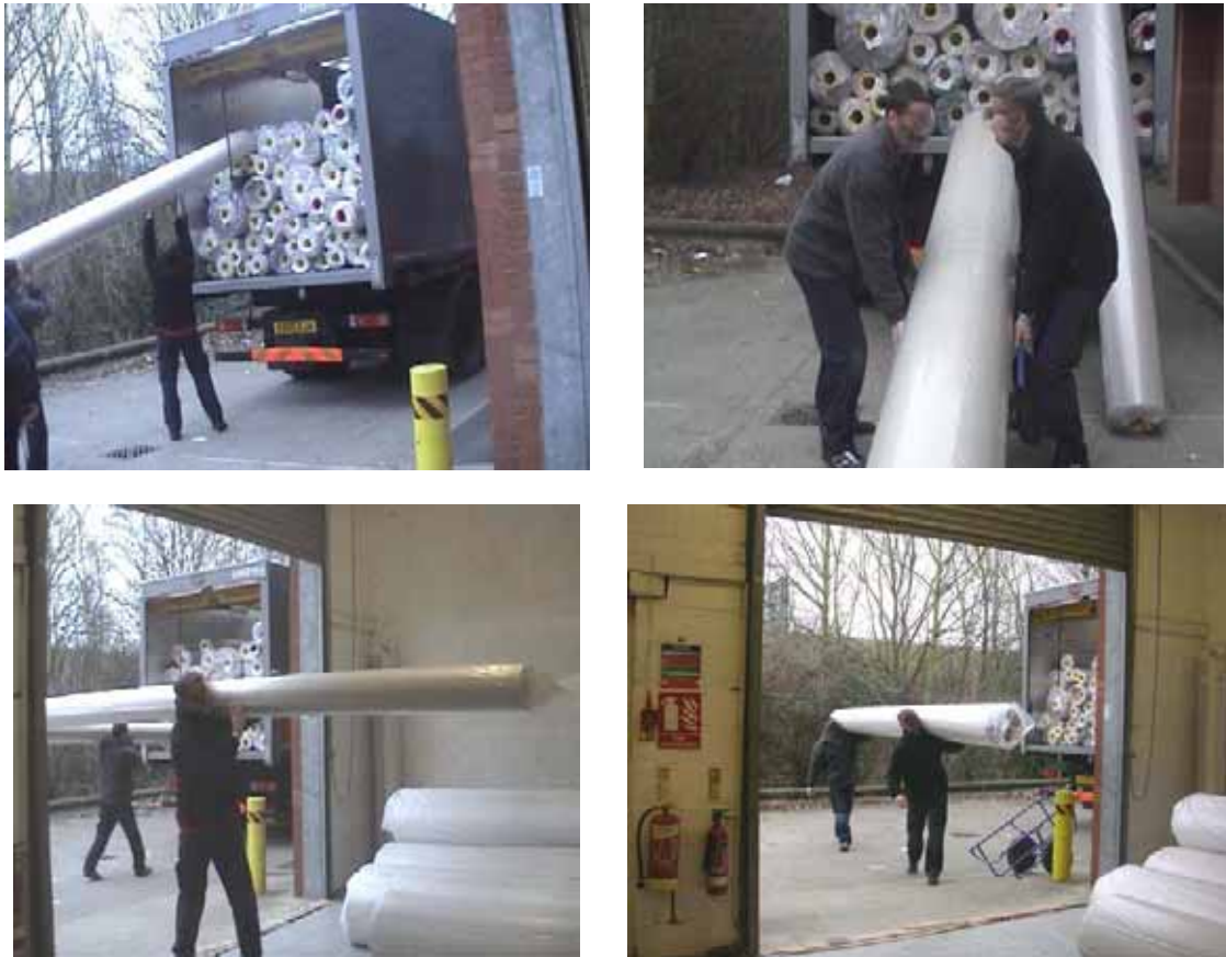
Figure 6. Typical handling activities when unloading a delivery vehicle without using a forklift and boom.
