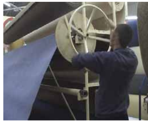
Figure 14. Winding on a new roll using carpet manipulator and wheel.
