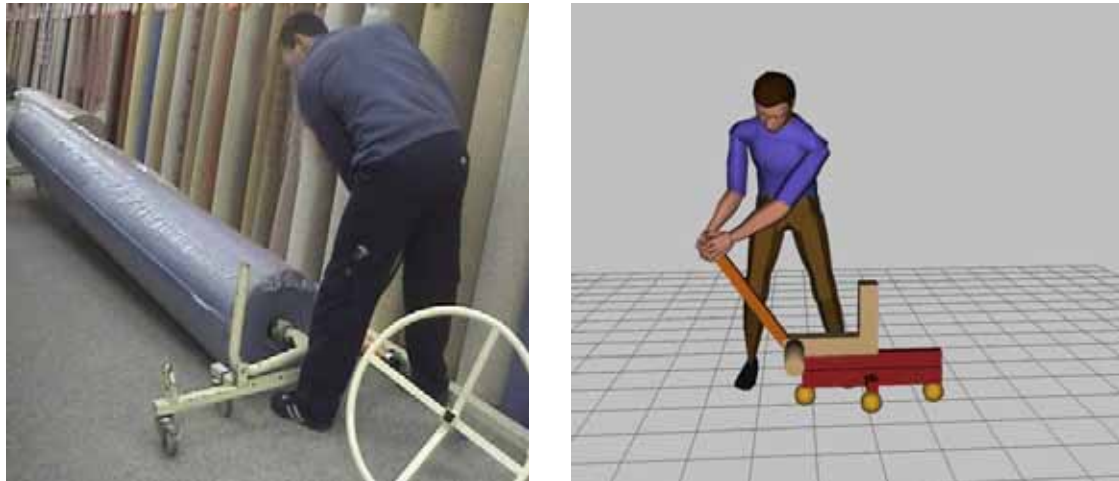
Figure 20. An example of using the carpet manipulator in the store and in the biomechanical model, during the initial lift on the manipulator lever arm.
