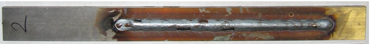
Fig 1. Weld carried out using HSL's Thermal Arc DC inverter
