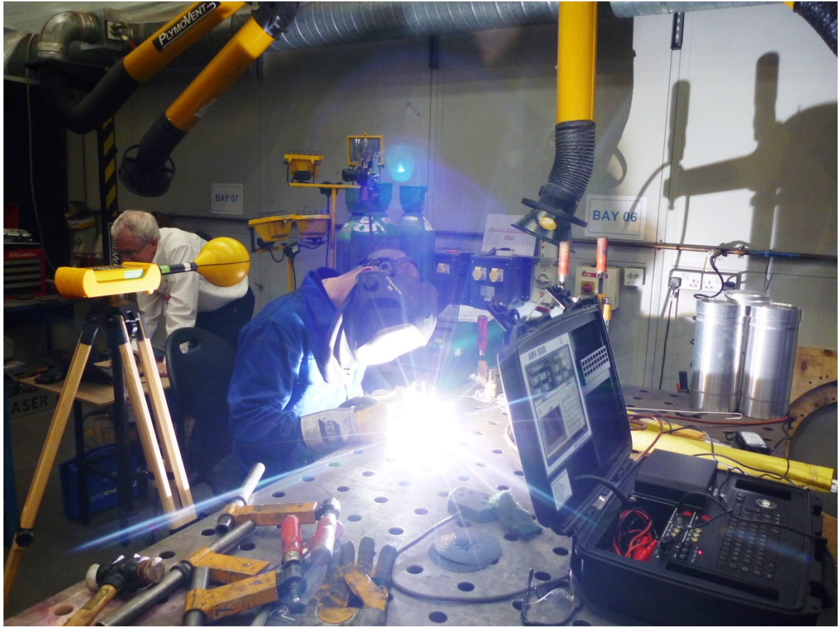
Figure B1 Measurement of magnetic field around arc welding processes.
