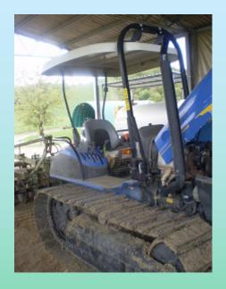
Cleaning of air filters is too difficult Lack of safe systems to hold the hood
