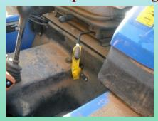
Safety device to allow movements only if the driver is at the controls
