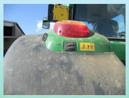
Tractor lift connection located at a too high position Poor visibility of the tow hook
