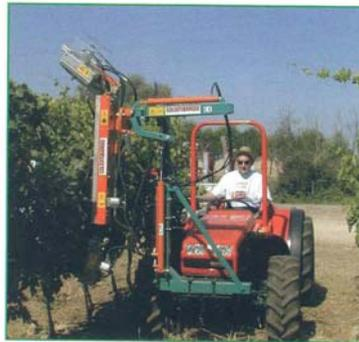
CIMATRICE DA VIGNETO A LAME ROTANTI: SPEEDY ROTOR
