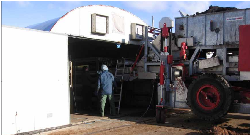
5 Filling machine used to lay compost in shelves
