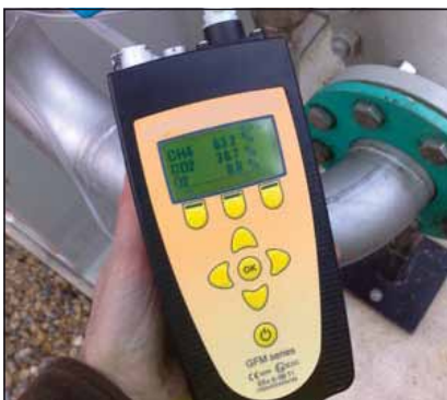
15 Carbon dioxide levels should be monitored and sheds ventilated accordingly
