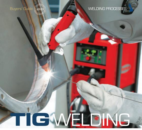
**TIG** welding (Tungsten Inert Gas), also known as GTAW (Gas tungsten arc welding), is where the welding arc is formed between a non-consumable tungsten electrode and the work piece with the weld being protected from atmospheric contamination by an argon, Argon + 2 to 5 per cent H2 or Helium and helium/argon inert shielding gas.
