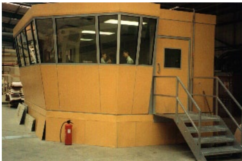
Figure 12 A noise refuge and control room
