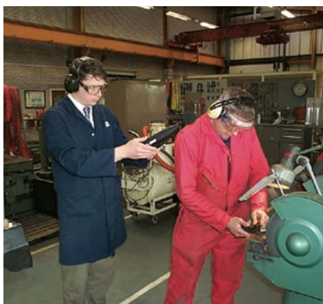
Figure 40 Making measurements with a hand-held sound level meter
