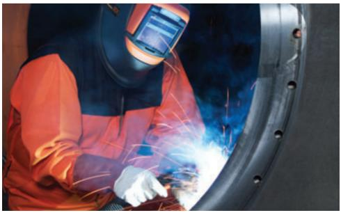
**MIG** (Metal Inert Gas)/MAG (Metal Active Gas) or Gas Metal Arc Welding (GMAW) is a welding process where an electric arc is created using a power supply between a continuous consumable metal welding wire and the workpiece.
