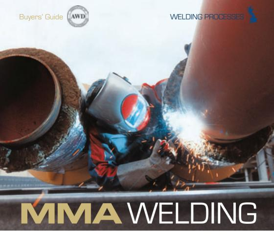
**MMA** (Manual Metal Arc) welding or SMAW (Shielded Metal Arc Welding) or sometimes known as Stick welding is a manual arc welding process that is the oldest and most versatile of the arc welding processes.
