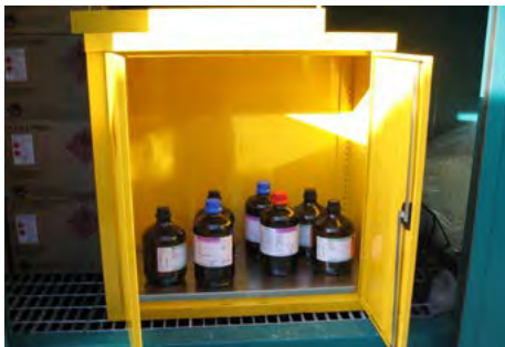
Inside a safety cabinet for flammable substances
