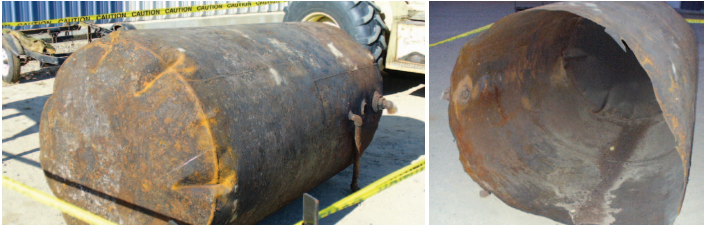
Exterior and interior views of the fuel tank involved in the hot work accident at A.V. Thomas Produce.
