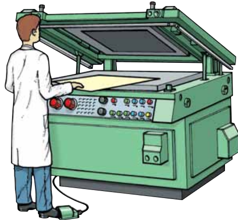
Figure 31 Hinged or clam-type screen printing presses with power closure should be fitted with safety trip bars
