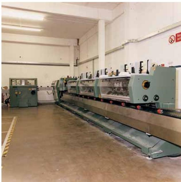
Figure 42 Fixed and interlocked guards should be provided for all dangerous parts of GSTs
