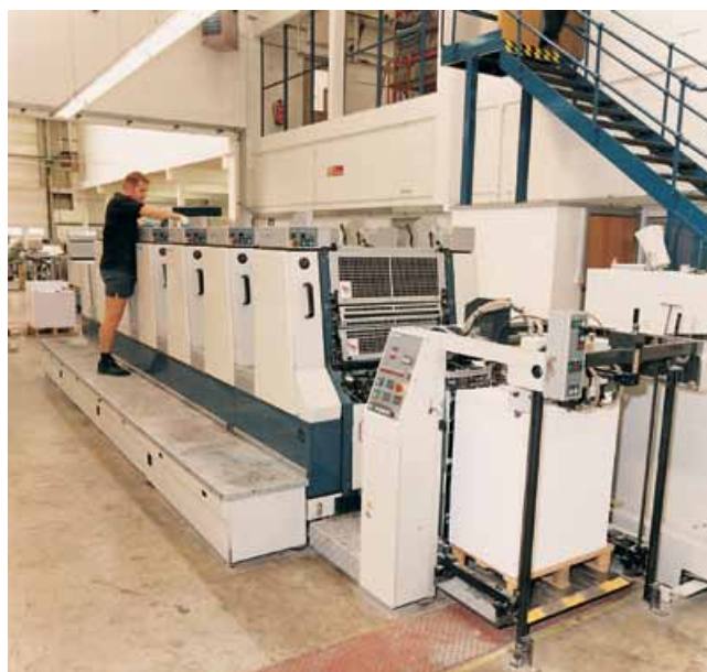
Figure 22 Emergency stop controls should be provided within reach of all operating positions
