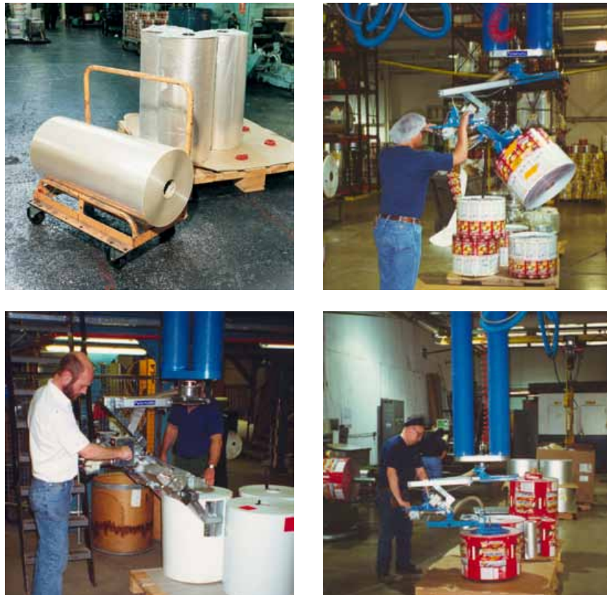
Figure 13 Reel and cylinder trolleys reduce the amount of manual lifting and carrying
