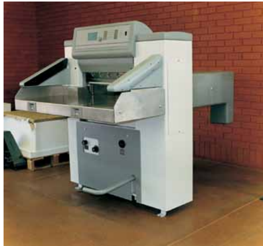
Figure 35 Guillotine fitted with photoelectric curtain and simultaneous two-hand controls
