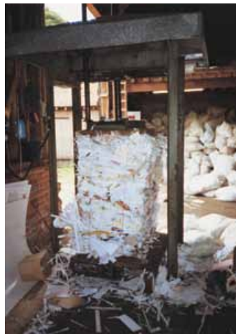
Figure 43 An unacceptable baling press
