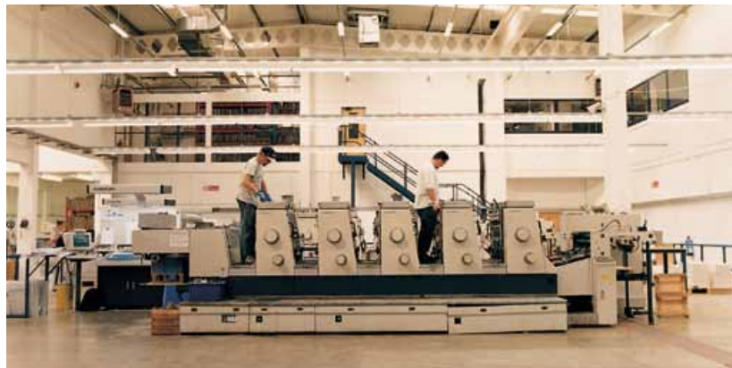
Figure 24 In multi-operator presses an audible pre-start warning device should be fitted
