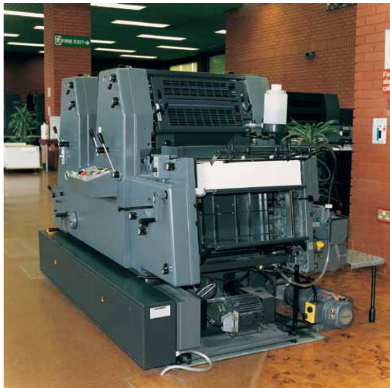
Figure 23 Two-colour press fitted with slotted, interlocked, all-enclosing guards
