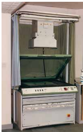
Figure 14 Screen all UV light sources adequately, preferably with automatic curtains or blinds
