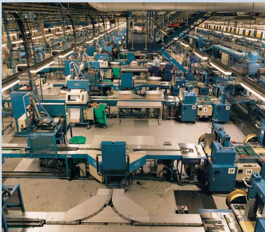
Figure 32 Conveyors, counters, stackers, tyers and strappers in publishing rooms need to be safeguarded
