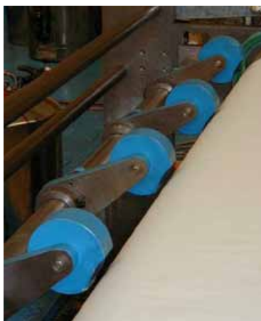
Figure 27 Propeller and slitter rollers should be guarded
