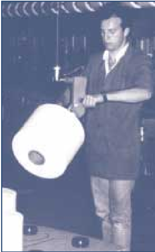
Figure 22 A mechanical lifting aid for packages of yarn
