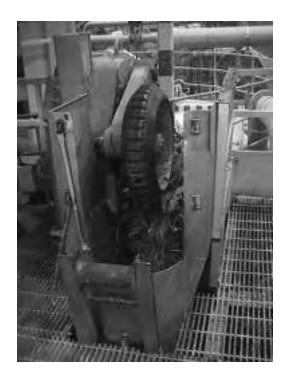
Figure 15 Ensure the guard is interlocked with both the movement of the capstan and the pneumatic system for operating the guillotine
