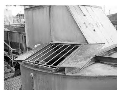
Figure 13 The fencing around open-topped pulpers should be designed so that people cannot climb onto it
