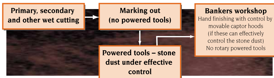
Figure 12 Segregation of dust-creating stonemasonry processes
