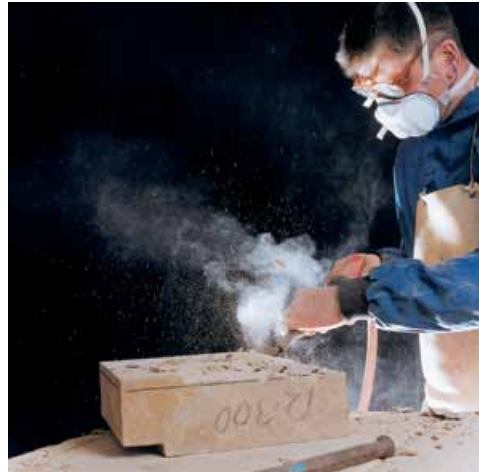
Photograph 11 Pneumatic chiselling on grit stone (see Figure 1 for likely crystalline silica content) can cause exposures up to 10 mg/m 3 respirable silica dust (see Figure 3). The respirator being worn would not protect the stonemason from this level of exposure.
