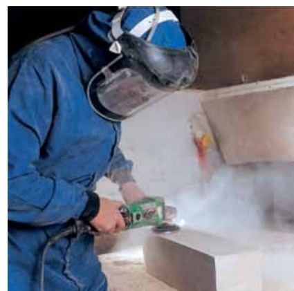
Photograph 7 Polishing dust control. Dust-laden radial air jets (top and see Figure 10) are too big and fast moving to be captured. Almost no control of stone dust by captor hood (top and see Figure 14) although quite effectively swept away within an exhaust ventilation booth (bottom and see Figure 15)
