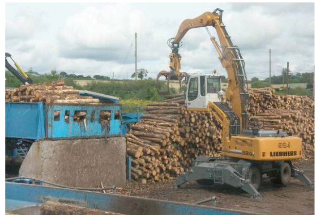
Figure 1 Feeding a sawmill by grabber
