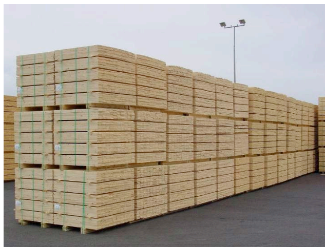
Figure 3 Well built stacks of banded sawn timber packs
