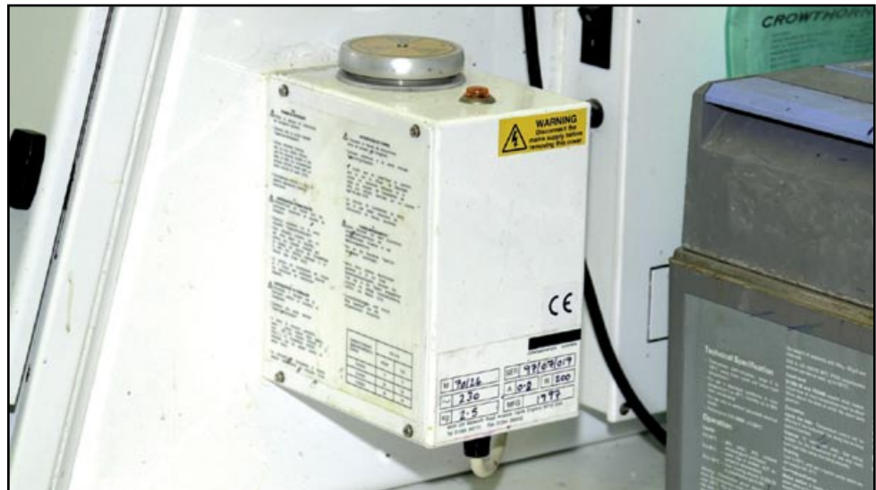
Figure 15 Device for fumigating cabinet
