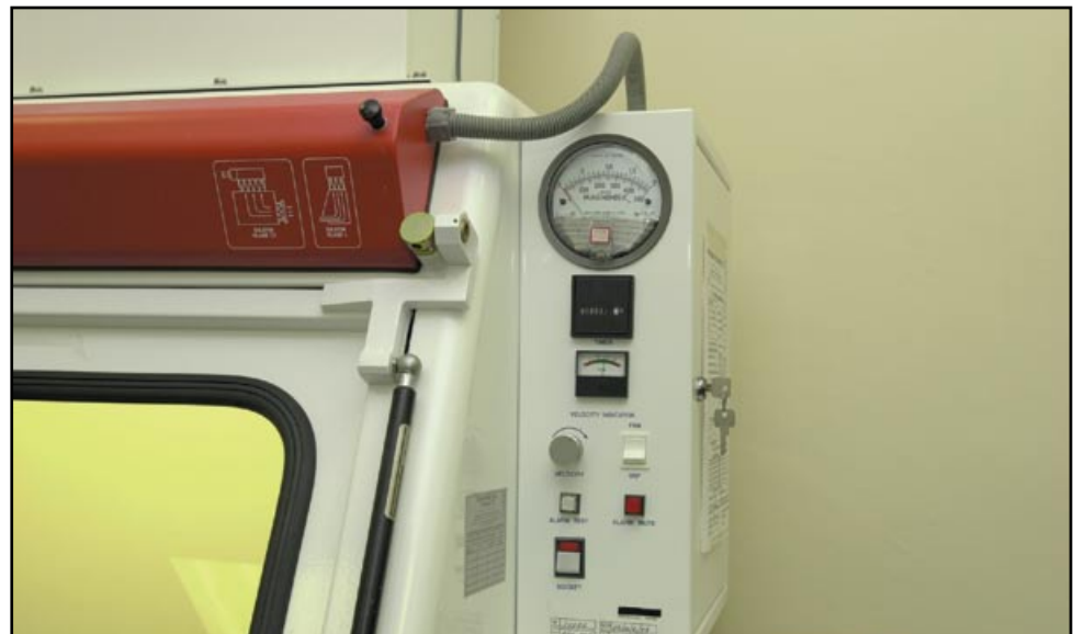
Figure 16 Alarms/indicators on safety cabinet
