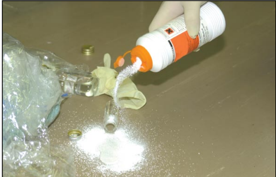
Figure 7 Clearing up a small liquid spill
