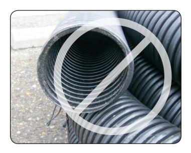
Do not use hoses with ridged or corrugated interiors (as shown) to vacuum wood dust.
