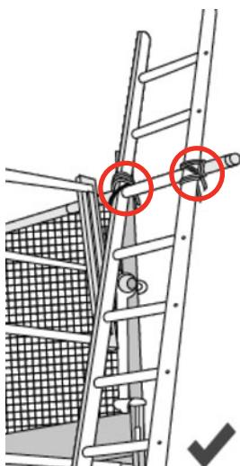
When using ladders to access another level, secure and extend the ladder at least 3 feet above the landing point to provide a safe handhold.
