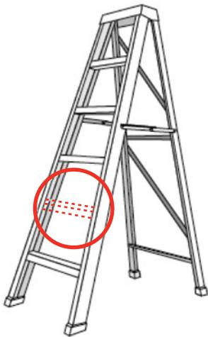
Do not use the ladder if the spreader bars do not have a locking device or mechanism.
