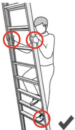
Maintain three points of contact with the ladder at all times.
