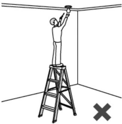
Do not work on the top rung of the ladder.
