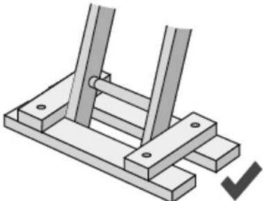
The base of the ladder should be secured.
