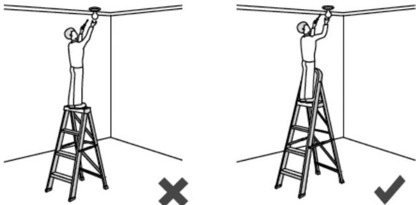
Use the right ladder for the job. For example, ensure the ladder is high enough for you to reach your work area without having to stand on the top rung.
