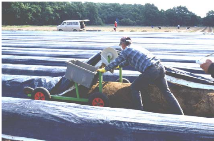
A simple harvesting system built by an individual grower. It is hand-moved, lifts the film from the ridge for several meters and contains a box to transport the harvested spears.
