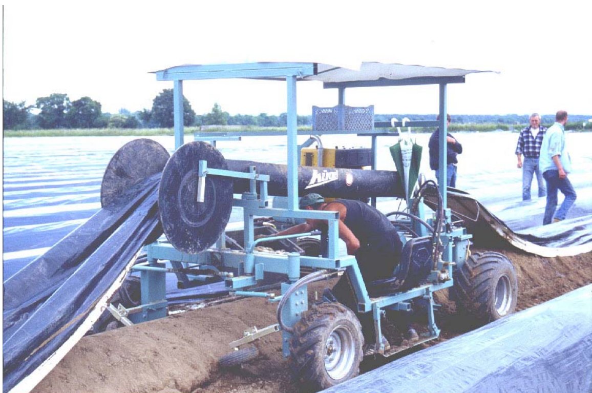
A commercial electrical-driven 1-row harvesting system with seat. The system lifts the film, transports the harvested spears, gives cover against sun and rain and takes care of the ridge.
