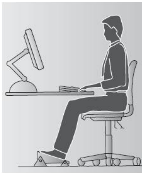
Figure 5.16 – Appropriate seated computer workstation arrangement using footrest
