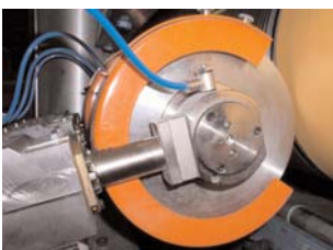
Figure 2 Slitter knife showing guarding
