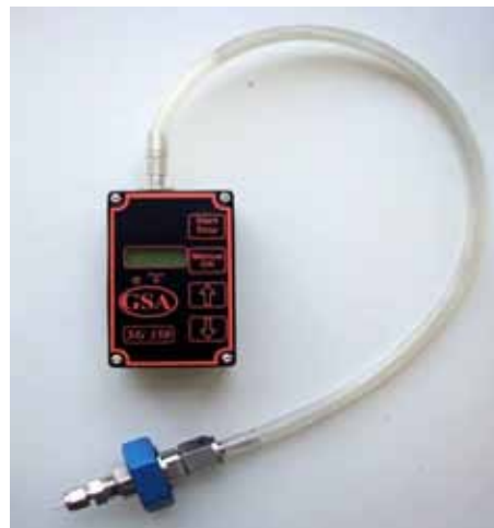
Figure 8. Pre-prototype CNT specific sampler by Fraunhofer IPA.
