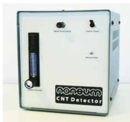
Figure 4. CNT detector developed by NANEUM
