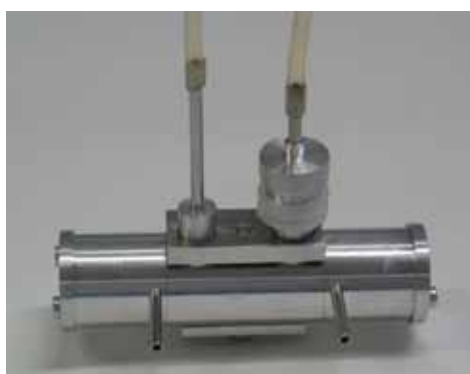
Figure 7. Extra-thoracic region (ETI) modular pre-separator developed by University of Lund
